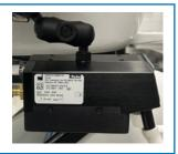
**7.** Run the white mixed gas tubing, clear vacuum tubing, and eAVS communication cable from the junction box up through the chair cantilever and out to the bag tee and eAVS.
