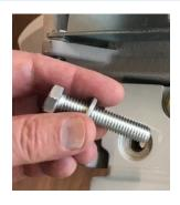
**2.** Replace existing bolt with the 2" bolt and existing split washer. Thread bolt through split washer and chair.
