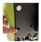
For PD2, GP2 and RS1 chairs, use the middle hole to mount the hardware.
