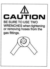
**Caution:** Make certain hoses are not crimped. Always **use two wrenches when tightening**, to assure that the Universal connectors are not loosened from the flowmeter cavities. Verify that the Universal connectors are tightened firmly to the flowmeter and that the DISS hoses are tightened firmly to the Universal connectors.
