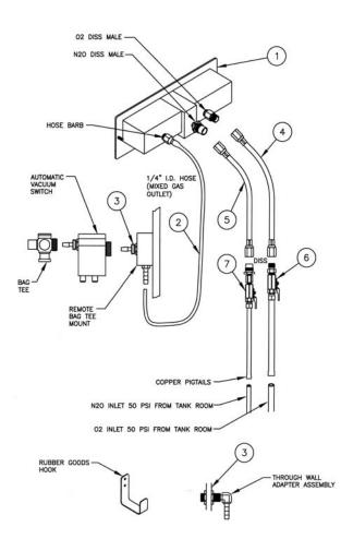
**INSTALL THE GAS LINES:** A qualified plumber can install the delivery piping up to and including the DISS Shut-Off Valves by following the details below and illustrations in this brochure.
