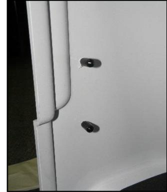
1. If holes are not pre-drilled, use LB-730 Plastic Template to align with Front Cover and mark hole locations and drill appropriate pilot holes or use the self-tapping feature of the included mounting screws (See Fig. 3.1).
